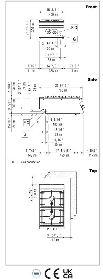
Modular Cooking Range Line EVO700 2-Burner Gas Boiling Top
